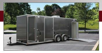
This ADA trailer features a hydraulic lift system to easily lower the unit to the ground
