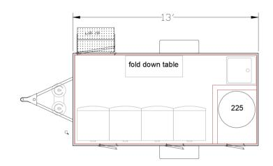
Dual propane tanks mounted on the tongue offer a self-contained water heating option.
